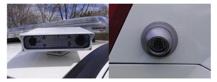
To use the system, operators need simply to select the appropriate zone within AutoVu, which includes the specific enforcement rules, and then drive through all areas of the zone. AutoVu will automatically scan and record all data pertaining to surrounding vehicles, compare that information to its database, and alert the operator if any vehicle is in infraction, requiring ticketing or other action.
